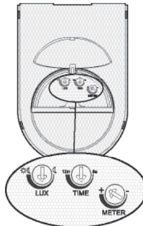
The sensor can be rotated horizontally within a 25° angle to modify the direction of detection.
