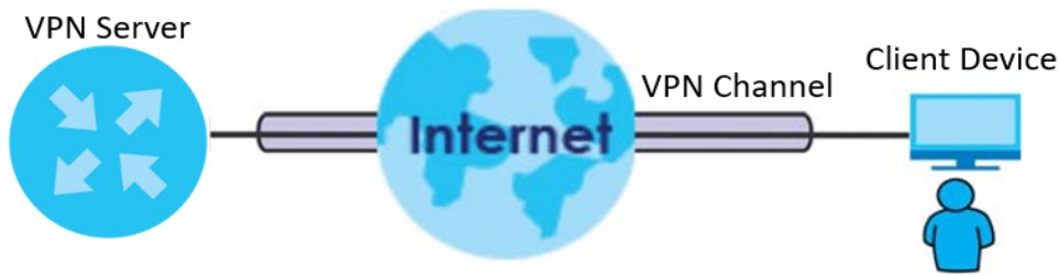
Figure 24 Example of NBG6818 Acting As VPN Server
