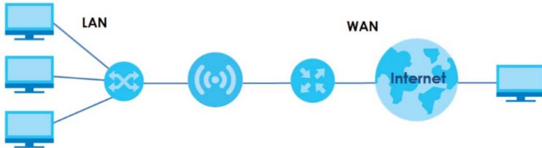
Figure 3 Internet Access Application: Ethernet WAN
