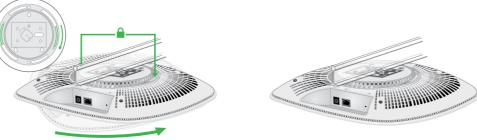
8. Twist the access point clockwise to lock it onto the mounting plate.
