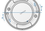
The screws **C** are now locked in their end positions **5** and the access point is fixed to the mounting plate.
