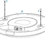
the attached screws C into the appropriate holes 3 of the mounting plate.
