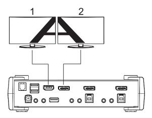
Note: The optimum resolution for two monitors in MST mode is 4K @ 30 Hz.
