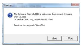
If you did not enable *Check Firmware Version*, the Utility installs the upgrade files without checking whether they are a higher level, or not.
