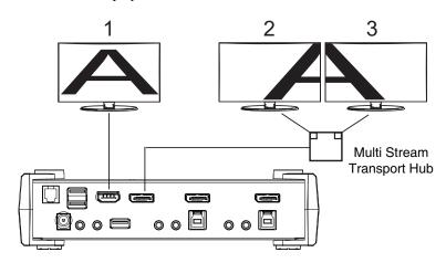
**Note:** In Splitter mode, the optimum resolution for each output is 4K DCI @ 60 Hz. If you connect an external MST hub to the CS1922M / CS1924M's DisplayPort port, the video resolution for the two monitors depends on the bandwidth shared between the displays.
