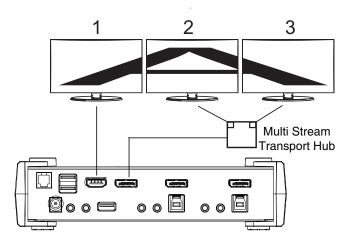
**Note:** The optimum resolution for three monitors in MST mode depends on the bandwidth shared between the displays.
