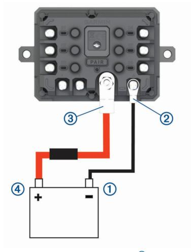
2 Connect the small ring end of the ground wire to the **GND** terminal ② on the device.
