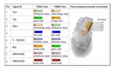
Though the device can be powered over Ethernet port it is not compliant with IEEE 802.3af-2003 standard. Powering RUT9xx from IEEE 802.3af-2003 power supply **will damage the device** as it is not rated for input voltages of PoE standard.
