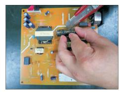
S20-2 Ensure cutting path within the glue, don't touch bulk cap. or PCB.
