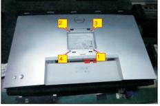
Tear off the screen protector, then wedge fingers between rear cover and the middle bezel on the corners of the top side of the monitor to release the rear cover, then use one hand to press the middle bezel, the other hand to pull up the rear cover in order of arrow preference for unlocking the rear cover.
