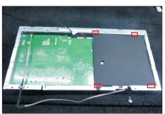
Use a Philips-head screwdriver to remove 8pcs screws for interface board and power board from the bracket.
