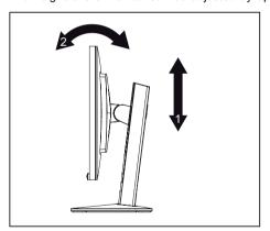
Hold the monitor with both hands on the right and left edge of the casing and move it up or down (1).
