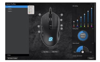
To switch profiles, first click on "Game Profiles" and then on the desired profile. The selected profile is immediately activated.
