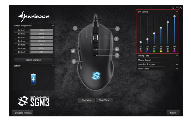
The DPI levels of the SKILLER SGM3 can be increased or decreased in six steps using the buttons with the DPI+ and DPI- functions. In the illustrated mouse in the software, these buttons are indicated with the numbers 6 and 7. In the menu "DPI Setting", the six preset steps can be individually modified.
