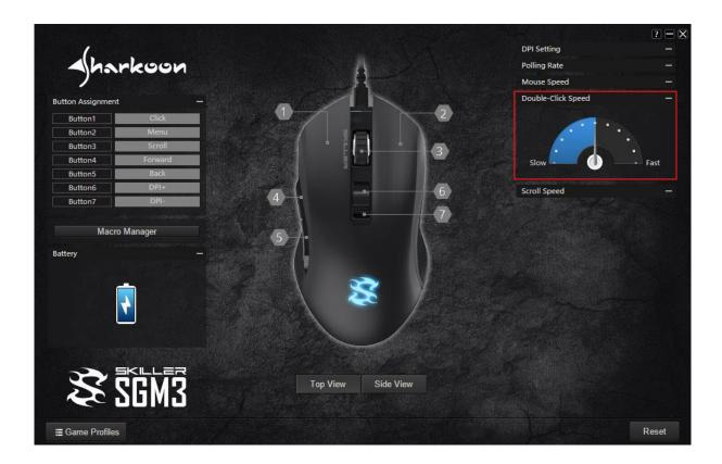
In this menu, you can set how far two mouse clicks are allowed to be apart while still being recognized as a double-click. The higher the value, the faster the clicks must follow each other. The double-click speed can be adjusted in eleven increments.
