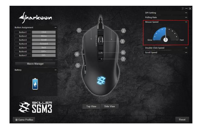
There are eleven steps to adjust the mouse speed. The higher the value, with the same mouse movement, the faster the cursor on the screen moves.
