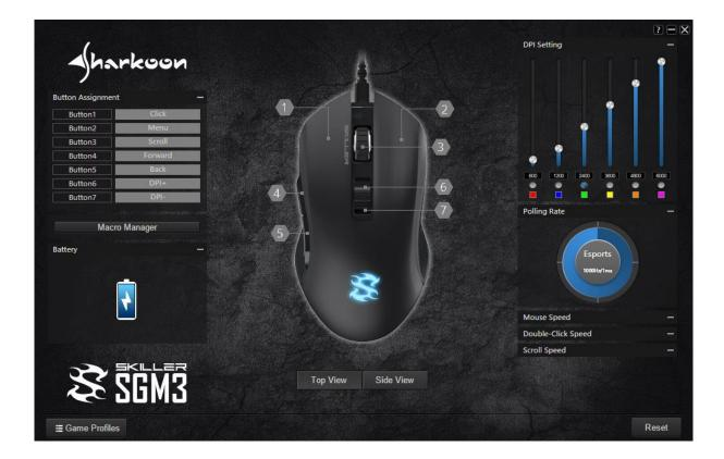
**DPI Setting:** In the menu "DPI Setting", the sensitivity of the mouse can be modified, and the illumination color of each of the six DPI steps can be selected.
