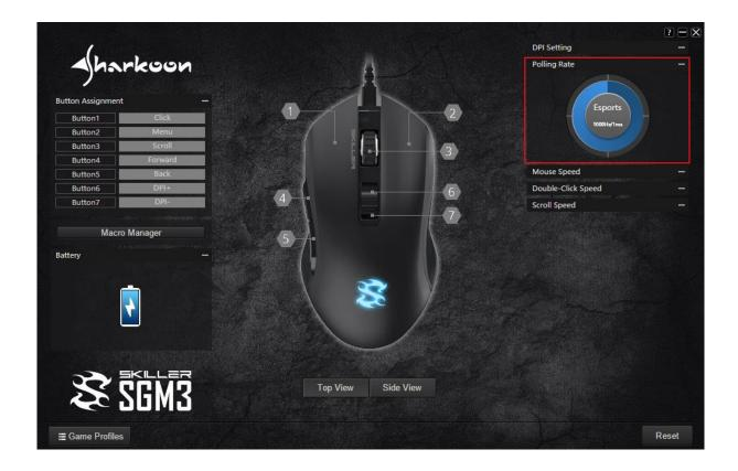
The circular diagram for changing the polling rate is divided into four quarters. Click on one of these quarters to activate the corresponding polling rate. The quarters begin with the lowest rate on the top left and run counter-clockwise to the highest rate on the top right. The following steps can be selected: Power-Saving (125 Hz, 8 ms), Office (250 Hz, 4 ms), Gaming (500 Hz, 2 ms) and Esports (1,000 Hz, 1 ms).
