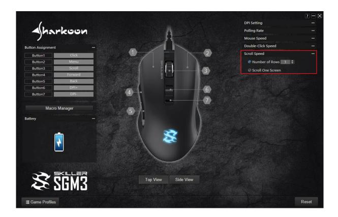
When scrolling, the mouse wheel moves the image to the selected number of rows or screen page. The standard setting is three lines. At a lower value, scrolling with the mouse wheel must be more frequent to achieve the same distance. With a higher value, less frequently.
