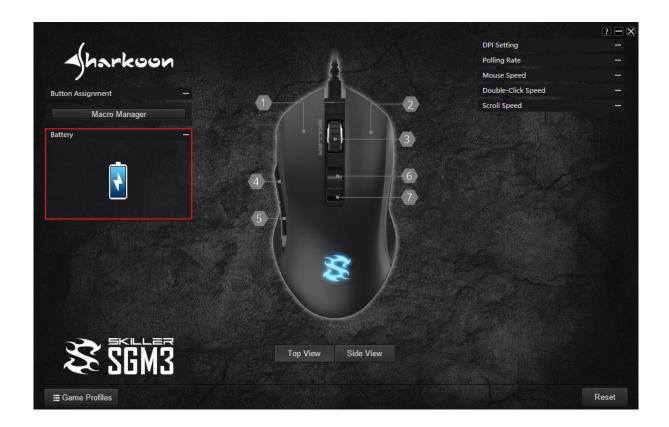
In this part of the software, the approximate battery charge of the SKILLER SGM3 is displayed in three levels. The illustrated battery is displayed as either full, half full or empty to indicate the current status of the battery.
