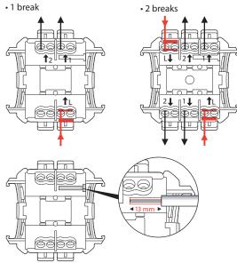
Type of terminals: automatic Terminal capacity: 1.5 mm<sup>2</sup> - 2.5 mm<sup>2</sup> (1 or 2 conductors) Stripping length: 13 mm
