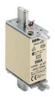
LV HRC FUSE LINK GL/GG WITH NON-INSULATED GRIP LUGS WITH FRONT INDICATOR SIZE 000, 100A, AC 500V/DC 250V
