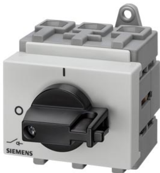
MAIN CONTROL SWITCH 3-POLE IU=63, P/AC-23A AT 400V=22KW BASE MOUNTING MOUNTING RAIL/TWO-HOLE MOUNTING KNOB BLACK
