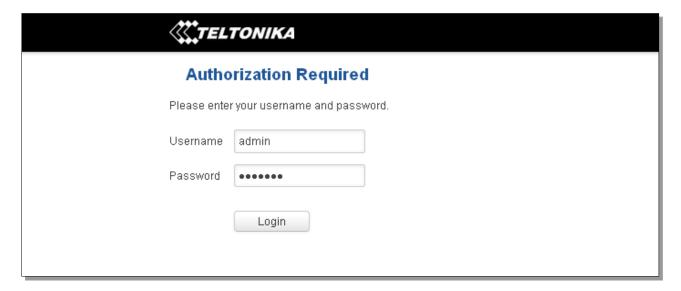
Enter the default password, which is "admin01" into the "Password" field and then either click Login with your mouse or press the Enter key. You have now successfully logged into the RUT240!
