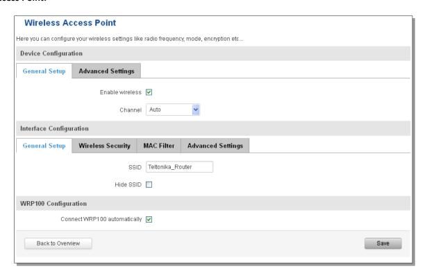
Here you can see the Overview of the wireless configuration. It is divided into two main sections – device and interface. One is dedicated to configuring hardware parameters, the other – software.
