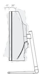
Tilting angle  $-5.0^{\circ}(\pm 2.0^{\circ}) \sim +20^{\circ}(\pm 2.0^{\circ})$
