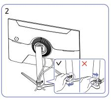
Pull the right side of the HOLDER-STAND CABLE to remove from the stand. The left side of the HOLDER-STAND CABLE can be damaged when pulled forcibly.
