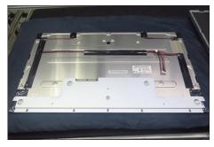
S20 Release the Mylar tape from the hooks of the main bracket.
