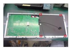
Use a Philips-head screwdriver to remove 10pcs screws for main board and power board, then disconnect the power switch wire from power board.
