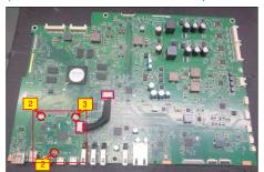
Take 2pcs EDP cables to connect with the main board, then connect the 2pcs cables of the power board with interface board. Turn over the interface board and locate it to the bracket. Use a Philips-head screwdriver to tighten 9pcs screws for locking the interface board and power board.
