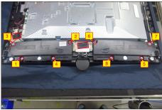
Connect 2pcs wires to 1pcs USB board, the locate the USB board into 1pcs bracket. Use a Philipshead screwdriver to tighten 1pcs screws for locking the USB unit and wire with the bracket. Take 1pcs cover to assemble with USB unit, and then fix the wires with 2pcs tapes as the picture below shown. (No.1 screw size=M3x5, Torque=4±0.5kgfxcm)
