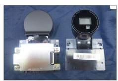
Tear off 1pcs aluminum foil for uncovering the fan, then use a Philips-head screwdriver to remove 3pcs S11 screws for unlocking the fan with the unit.
