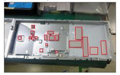
S2 Take 1 pcs master switch to assemble with the main bracket chassis as the picture below shown.
