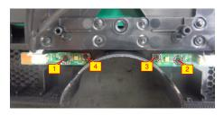
Release the front bezel away from the middle frame, and put the front bezel on a protective cushion, then tear off the black mylar tape and release LED board from the hooks of the front bezel, then release the touch board from front bezel by tearing off the tape.
