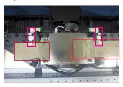
Take two speakers to locate into the probers of the middle frame, then connect the two speakers wires and fix the wire on the frame with 1pcs acetate tape. Connect the speaker wire to the main board and fix with 1pcs tape. Use a Philips-head screwdriver to tighten 8pcs screws for locking two speakers.
