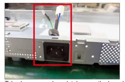
Take 1pcs power board, take over the board and put it into the bracket chassis, then connect the switch wire to the power board. Use a Philips-head screwdriver to tighten 1pcs screw for locking the grounding wire with the bracket.
