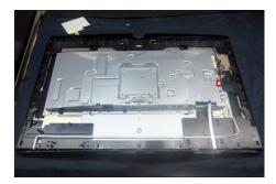
Tear off all the tapes for releasing the LED wire and touch wire, then tear off 2pcs rubber pads. Use a Philips-head screwdriver to remove 4pcs screws for unlocking the left and right DMic boards, then tear off the left and right DMIC boards from the middle frame. (No.1~4 screw size=M2x2.4, Torque=1±0.2kgfxcm)
