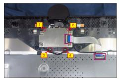
Paste 2pcs mylar tape to cover the camera unit, then paste 2pcs aluminum foil on the specific position as the picture below shown.
