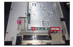
lift up the main bracket and then disconnect the twoEDP cables away from the connector of the panel, then take away the main bracket and put it aside.
