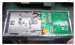
Take 1pcs main board, 1pcs 1pcs TBT modular board, then connect the TBT board to the main board.
