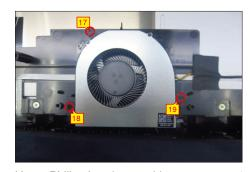
Use a Philips-head screwdriver to remove 16pcs screws for unlocking the middle frame with the panel, then tear off 3pcs tapes and disconnect fans' wire and touch wire from the connectors, and then remove the fan from the hook of the middle frame.
