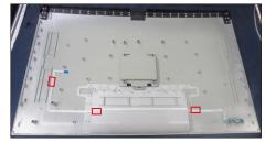
Move the assembled rear cover close to the panel unit, then connect the joystick key cable to the connector of main board.
