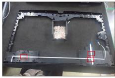
Take 2pcs DMIC boards(left and right) and some essential wires. Connect the left and right DMIC boards with wires, and tear off release paper and paste the two boards to the hooks of middle frame, then use a Philips-head screwdriver to tighten 4pcs screws for locking the Mic boards with middle frame. Paste 2pcs rubber pads on the correct positions of two DMIC boards by tearing off the release papers. (No.1~4 screw size=M2x2.4, Torque=1±0.2kgfxcm)
