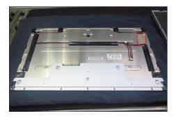
Move the main bracket chassis close to the panel, then connect the two EDP cables to the connectors of the panel.
