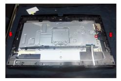
Take 1pcs bracket cover to assemble with the bracket, then use a Philips-head screwdriver to tighten 4pcs screws for locking the cover with the bracket. Use the screwdriver to tighten 4pcs screws for locking the main bracket with the panel.
