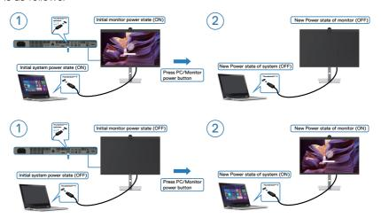
When the monitor and PC power state are both ON, while you **press and hold 4 seconds on monitor power button**, the screen prompt will ask if you would like to shut down the PC.
