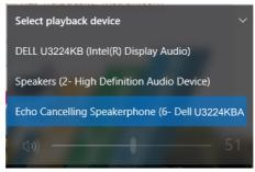
If only the HDMI or mDP cable is connected from your monitor to the computer, only one speaker named **DELL U3224KBA** from the monitor will show in the **Sound** setting interface.
