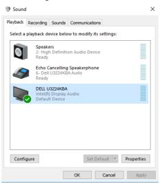
If the USB cable and the HDMI or mDP cable are connected from monitor to the computer, two audio paths named **DELL U3224KBA** and **Echo Cancelling Speakerphone U3224KBA** from the monitor will show in the **Sound** setting interface. The **U3224KBA** monitor would show options for two audio paths supported in the monitor.
