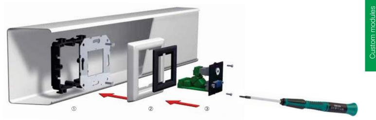
The mounting box is inserted into the trunking. This forms the base onto which the mounting plate<sup>①</sup> and adapter frame<sup>(2)</sup> (50x50 mm or 55x55 mm) and the Bachmann custom module are bolted<sup>(3)</sup>.
