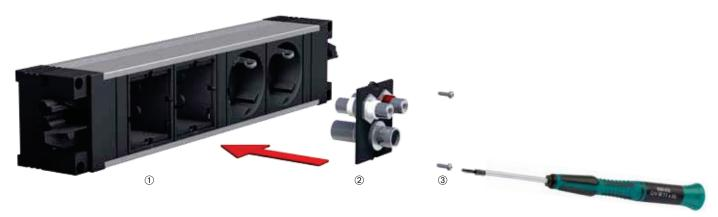
The empty built-in frame<sup>①</sup> of Bachmann facility systems accommodates the custom modules<sup>②</sup>, which are fixed in place with two Torx screws<sup>③</sup>. The custom modules can be easily exchanged by loosening the screws.
