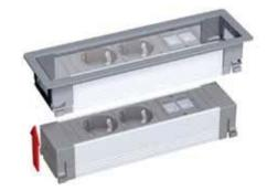
Built-in frame for desk/table top thicknesses:from 10 mmInstallation depth (of built-in frame):approx. 36 mmCorner radius for flush mounting:R5Total installation depth (with cables):approx. 70 mm
