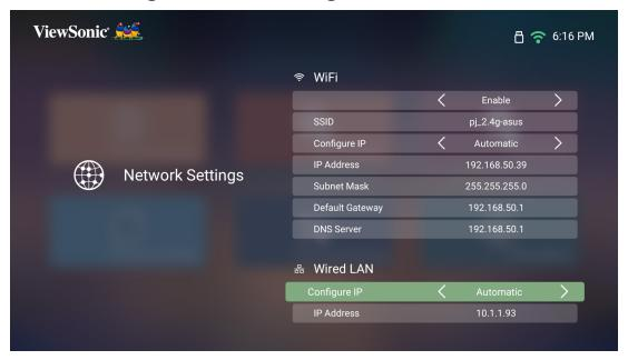
**3.** You can Configure the IP automatically or manually. Choosing **Manual** will allow access to **IP Address**, **Subnet Mask**, **Default Gateway**, and **DNS Server**.
