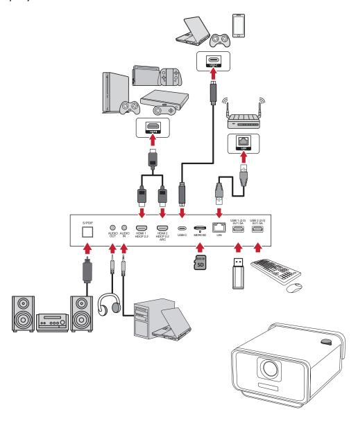
The projector will automatically search for input sources. If multiple sources are connected, press the **Source** button on the remote control to select the desired input, or press the **Down** button when at the **Home Screen** until the source list is displayed.
